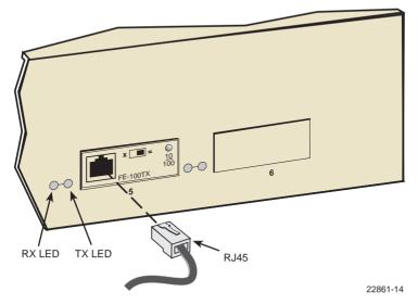
Figure 3-9 FE100-TX Port Connection
